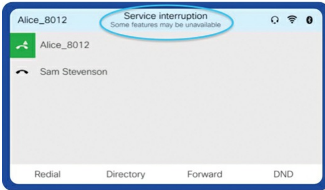
Figure 6-16 IP Phone Indicating It Is Registered to a Survivability Gateway
